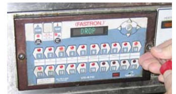
Figure 1: Remove the existing controller.
