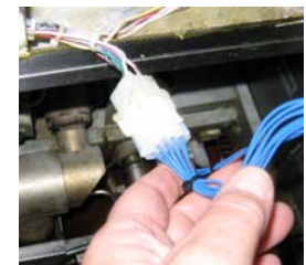
Figure 2: Connect the F3000 using the supplied harness.
